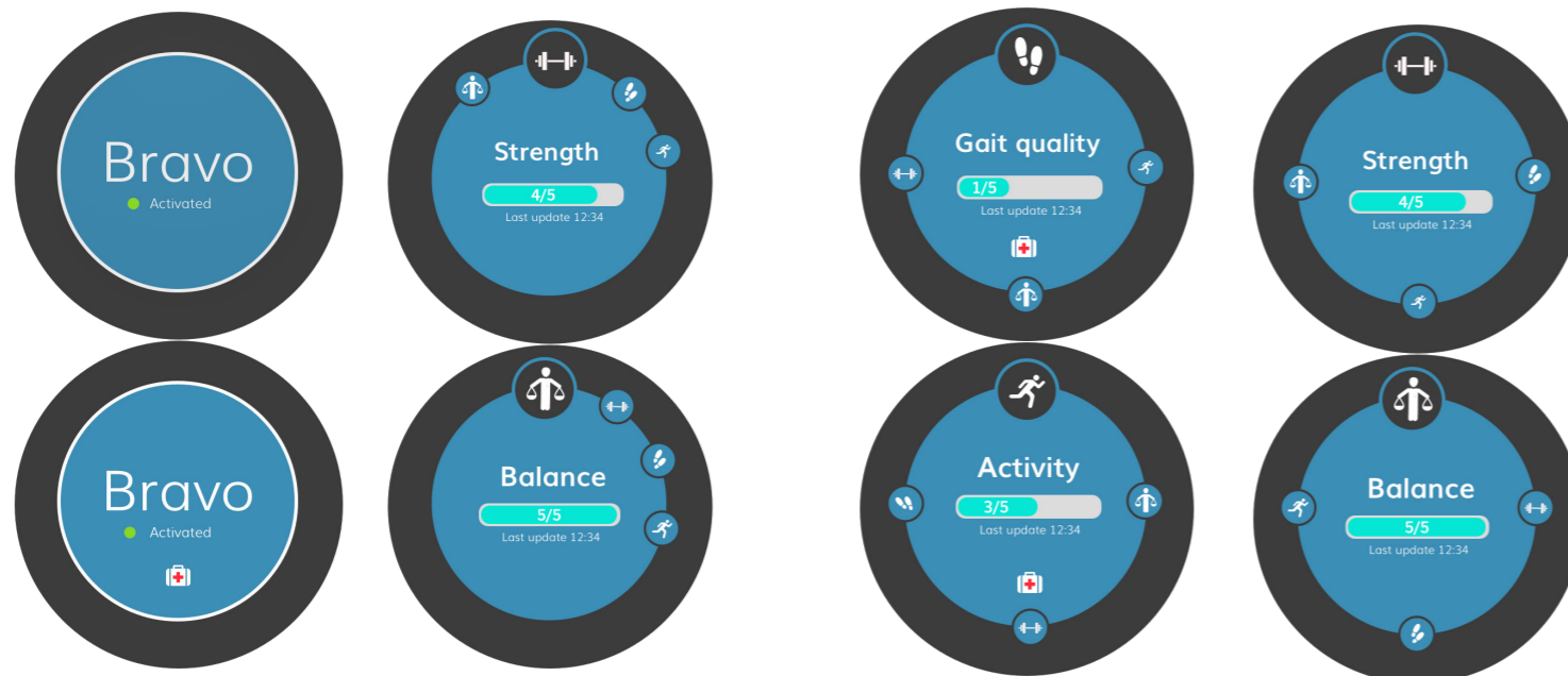
Iteration 1 Too complicated for the user to rotate back and forth through the categories, they wanted to continue with rotating the element.
